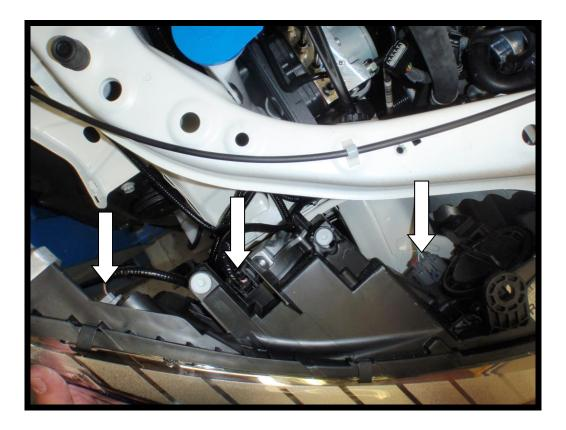
21. With the bumper and headlight removed you will now need to remove the inlet pipe. Undo the hose clip and pull away from the pipe, undo the four bolts holding the pipe work in position and one bolt at the back holding the inlet pipe in position. Remove the small rubber hose to the left.
