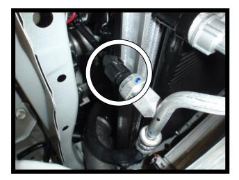
24. Unclip the vacuum hose, undo the three bolts and remove the dump valve.
