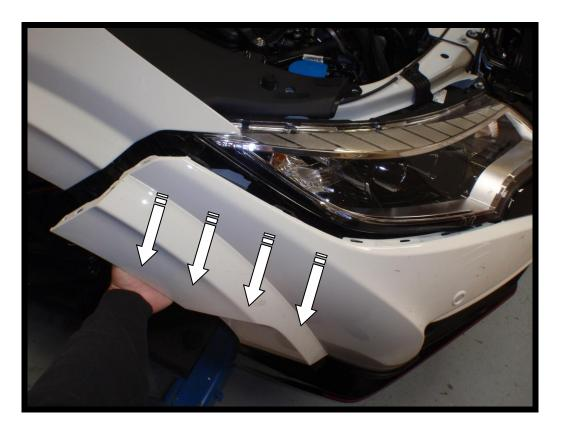
16. With the sides of the bumper pulled out unclip the spot lights and parking sensors.
