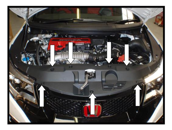
9. *Please note the following Steps 9 - 12 are not necessary if you are fitting the supplied blanking plate.* Unclip the vacuum hose leading to the dump valve and remove the small boost hose.
