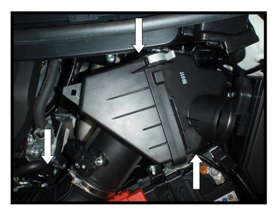
3. With the filter now removed undo the hose from the cast aluminium pipe.
