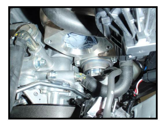
25. Install the planking plate and refit the inlet pipe in reverse order of removal.
