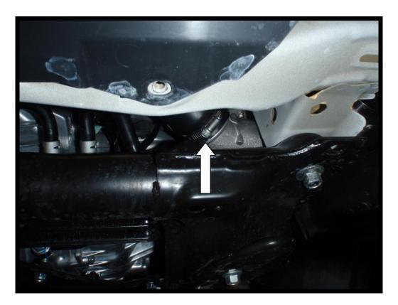
7. Attach the dump valve to the hose with the vacuum port facing down. Install the new silicon hose making sure there is clearance around the dump valve and attach with the clips supplied in the kit.
