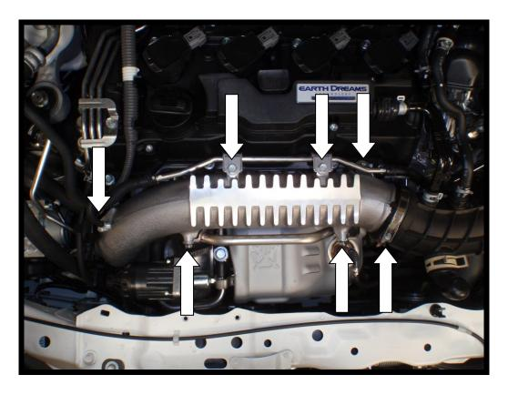
22. Undo the two bolts holding the plastic clip in position and move it as far out of the way as possible. Undo the two bolts from the flange of the pipe and remove.
