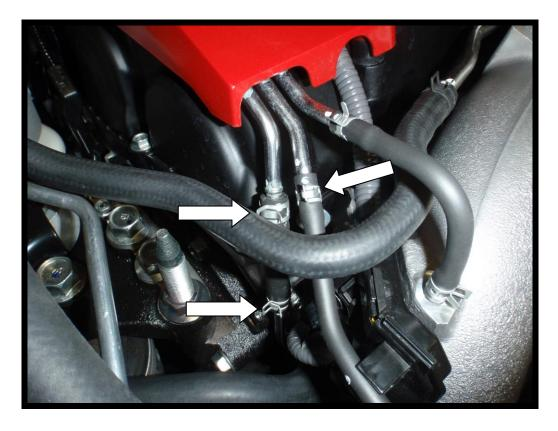
10. Using the short pieces of silicon hose make a loop with a t-piece in it and connect the vacuum hose leading to the dump valve. This will keep the OEM dump valve permanently shut.
