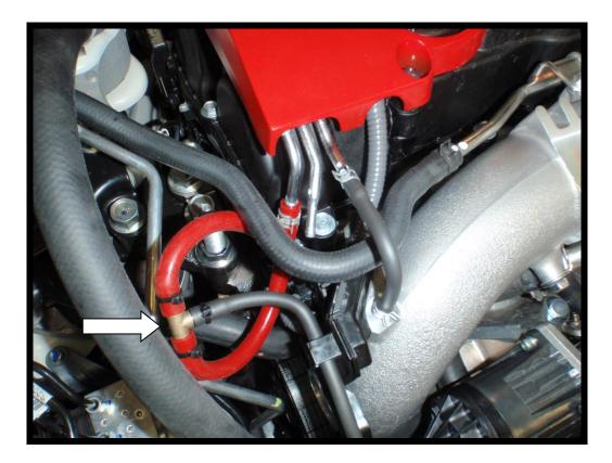
11. Connect the longer length of silicon hose to the vacuum source.
