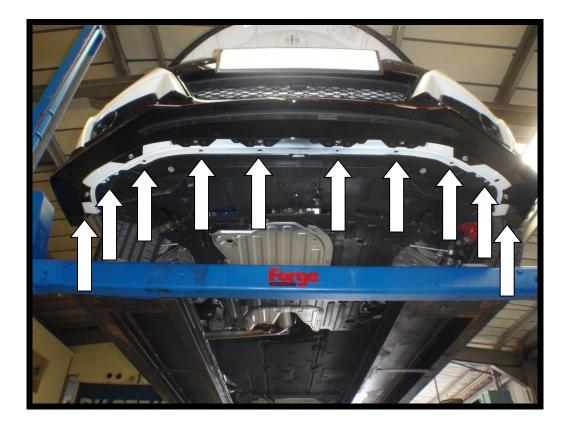
15. Pull the bumper out from the wing and the head light. Take care of the arch as it is only stuck with double sided sticky tape and can easily detach from the bumper.
