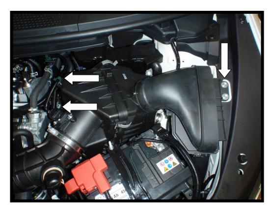
2. Undo the clip on the rubber hose and undo the two bolts on the filter box, pull the filter box upwards to remove from the vehicle.
