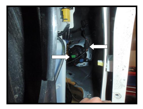
17. Undo the two bolts at the front of the bumper, the bumper is now free to remove.
