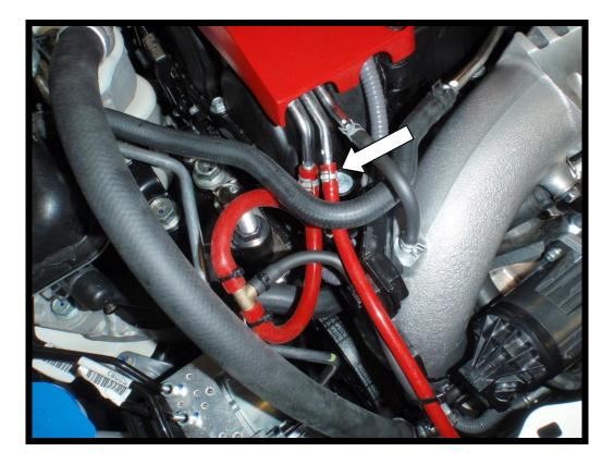
12. Feed the silicon hose through the slam panel, across the radiator and back to the new dump valve.
