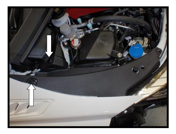
19. Undo the two bolts from under the headlight and pull the headlight forward.
