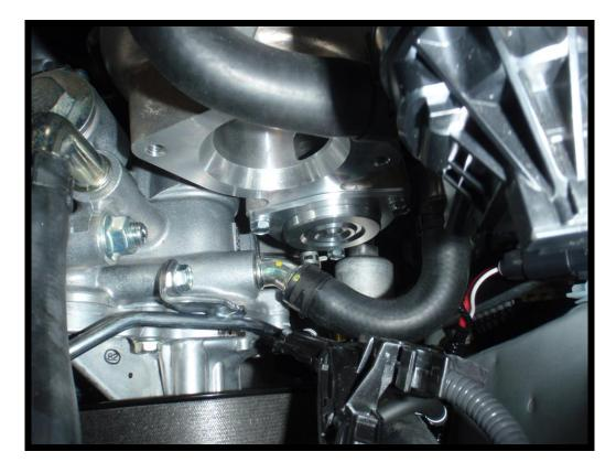
26. Connect the vacuum hose to the long length of silicon hose and joiner supplied in the kit. Feed the silicon hose through the slam panel, across the radiator and back to the new dump valve.
