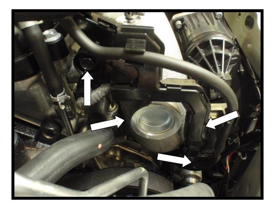
23. To gain excess to the dump valve remove the rubber ducting and unplug the air conditioning.
