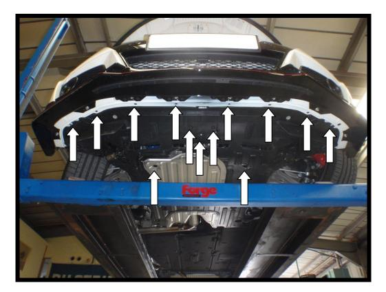
5. There is a second under tray which also needs to be removed undo the two clips and pull out the under tray.
